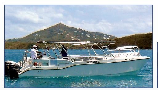
LENGTH: 35'5" WP 34'6" APPROX WEIGHT: 7500 LBS BEAM: 12' HORSEPOWER MAX CAPACITY: 2X300 HP FUEL CAPACITY: 2X80 GAL OR 2X111 GAL
