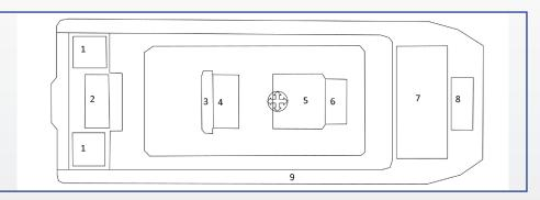
1 ACCESS HATCH 2 BAIT WELL 3 FLIP-FLOP SEAT 4 FUEL TANK 5 CONSOLE 6 SEAT WITH STORAGE 7 FISH BOX 8 ANCHOR LOCKER 9 RAIL
