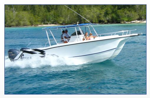
LENGTH: 29'1" APPROX WEIGHT: 5500 LBS BEAM: 9'8" HORSEPOWER MAX CAPACITY: 2X115-2X250 HP DRAFT: 13" FUEL CAPACITY: 2X80 GAL
