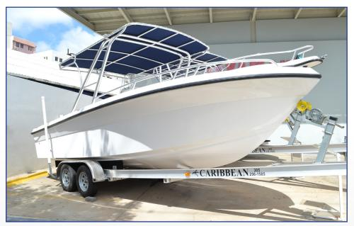
LENGTH: 22' APPROX WEIGHT: 3000 LBS BEAM: 8'6" DRAFT: 17" HORSEPOWER MAX CAPACITY: 250 HP FUEL CAPACITY: 57 GAL
