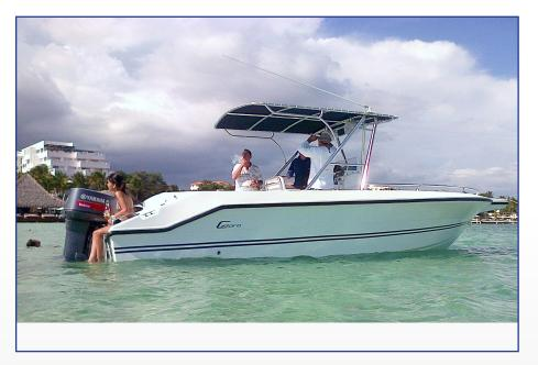
LENGTH OVER ALL: 26' APPROX WEIGHT: 4000 LBS DRAFT: 1' 5" BEAM: 8' 6" HORSEPOWER MAX CAPACITY: 2X250 HP FUEL TANK CAPACITY: 80 GAL
