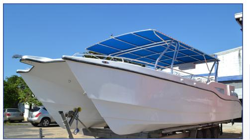
LENGTH: 35'5" WP 34'6" APPROX WEIGHT: 7500 LBS BEAM: 13' HORSEPOWER MAX CAPACITY: 2X300 HP FUEL CAPACITY: 2X80 GAL OR 2X111 GAL
