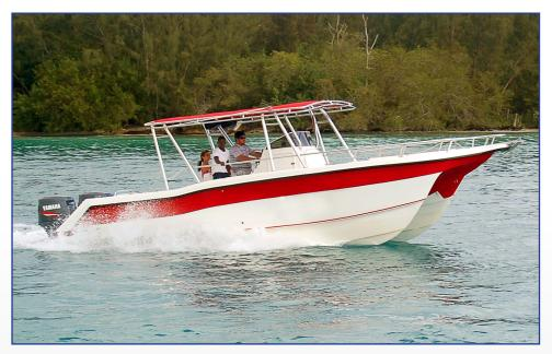
LENGTH: 30' APPROX WEIGHT: 6000 LBS BEAM: 9'8" HORSEPOWER MAX CAPACITY: 2X115 HP-2X250 HP DRAFT: 13" FUEL CAPACITY: 2X80 GAL
