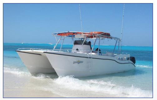
LENGTH: 35'5" WP 34'6" APPROX WEIGHT: 7500 LBS BEAM: 12' HORSEPOWER MAX CAPACITY: 2X300 HP FUEL CAPACITY: 2X80 GAL OR 2X111 GAL
