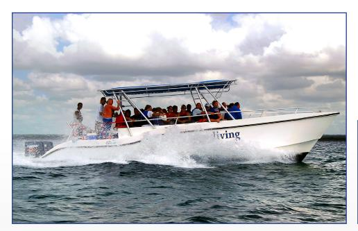
LENGTH: 35'5" WP 34'6" APPROX WEIGHT: 8000 LBS BEAM: 12' HORSEPOWER MAX CAPACITY: 2X300 HP FUEL CAPACITY: 2X80 GAL OR 2X111 GAL
