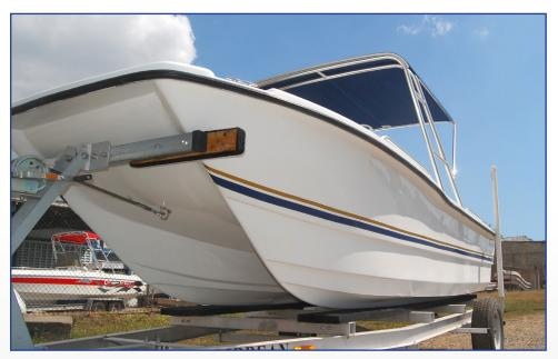
LENGTH: 17'10" APPROX WEIGHT: 1600 LBS BEAM: 7'2" HORSEPOWER MAX CAPACITY: 115 HP DRAFT: 10" FUEL CAPACITY: 20 GAL
